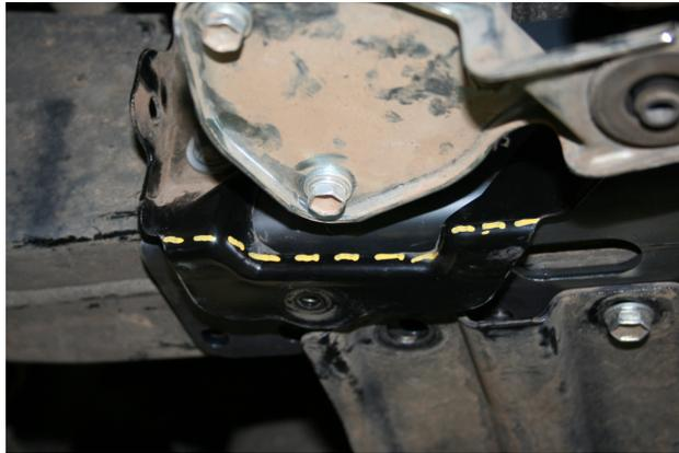
5. Fit Kaymar wing brace between compressor bracket and chassis. Secure using M8 x 20 bolts, M8 spring and flat washer.
